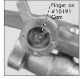
Make sure the #10191 cam is correctly keyed into the slot on the drive arm shaft. Notice the correct orientation of the finger on the cam for proper arm operation.
