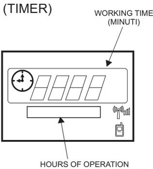
To set the the minutes (minimum 1' max 1440') of running of the motor pump after the command:
