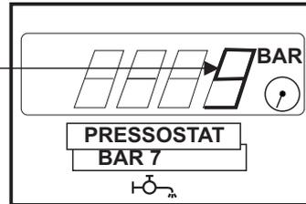
Press to select the pump water pressure gauge
