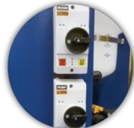
▶ Features single or dual configuration, motor starter protection preset to FLA of each motor. One switch controls the Agitator motor and the other controls the Pump.
