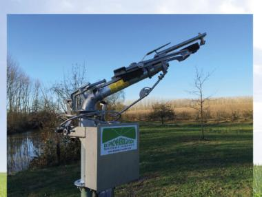
No program is necessary, the Gun Corner is a device at the front of the irrigation.
