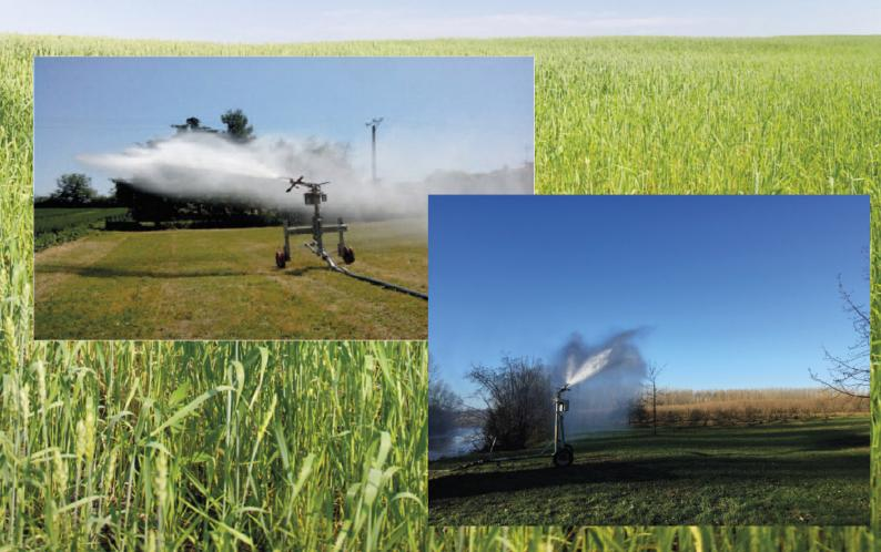
It makes it possible to bring the starting positions of the Gun Corner to 15 meters from the edge of the plot avoiding splashing water outside of this one.
