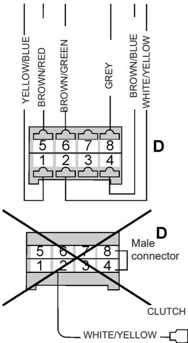
To connect PUMP PRIMING, remove the male connector, insert the connector with the wires brown/blue yellow/blue.
