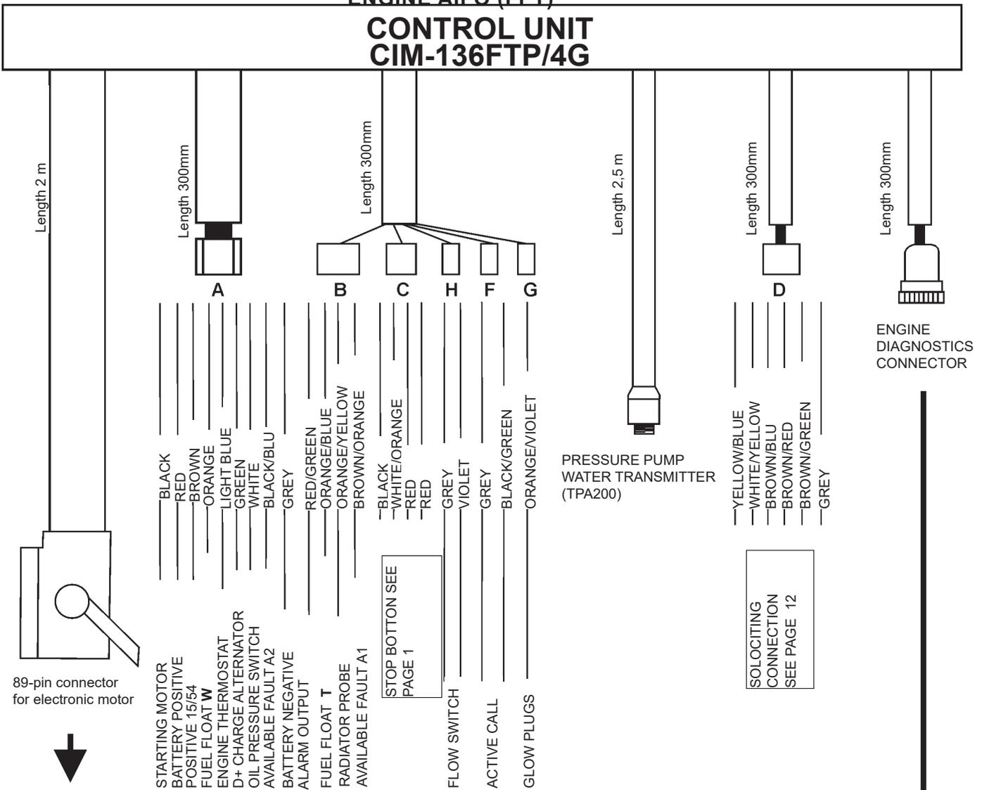
**Pin arrangement of 89-pin connector.**
