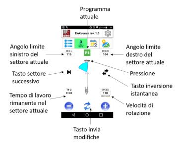
In order to change the limit angles of the current sector or the rotational speed touch the pane you are interested in, modify the value with the button + and – until the desired value and finally touch the central confirmation button. Immediately, the new values are sent to the raingun which immediately changes the current irrigation sector and the rotational speed will change after the first reverse of rotation.
